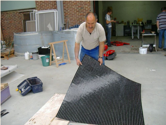
A suitably constructed mosaic panel can bend.
